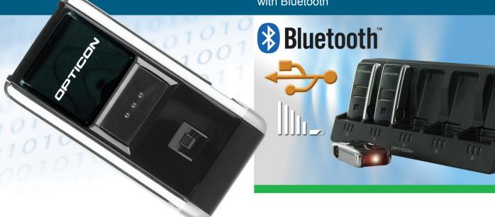
The OPN 2002 Bluetooth memory scanner combines convenient barcode data collection with flexible communication options. The device allows storage and removal of barcode scans. The final collection can be transmitted by cabled or wireless interface, both options are provided.
