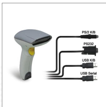
Cable replacement solution for Legacy Output (PS/2 keyboard, RS 232, USB keyboard and USB Serial)
